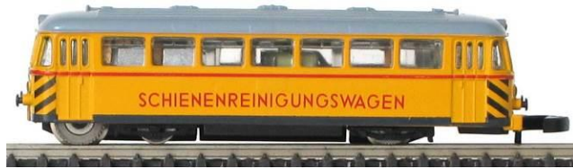
8802 – Track Cleaning Locomotive Two of the three axles on the track cleaning car are powered. The wheels on the rear and front axles are grooved. The cleaning wheels on the front axle turn faster than the wheels on the inner and rear axles, thus causing dirt to be thrown off of the track.
