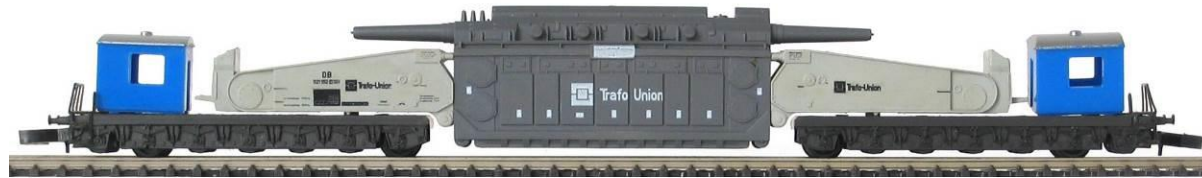
8620 – Depressed Center Flat Car (qty 3) Trafo Union Schnabel Car - loaded with transformer.
