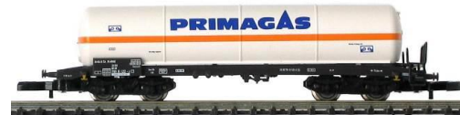
82180 – Gas Tank Car without Heat Shield Private car of "PRIMGAS GmbH" company, Krefeld. Registered with German Federal Railroad (DB).
