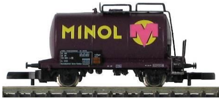
8203 – Petroleum Oil Tank Car Car privately owned by Minol Petroleum Oil Distribution, Inc., Berlin, Germany. Used on the German State Railroad (DR) of the GDR.
